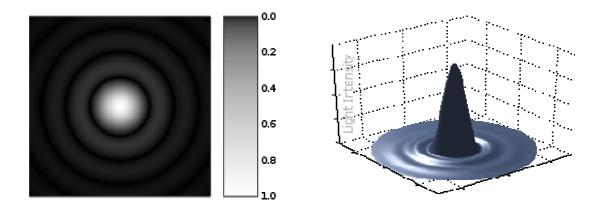
We can now go on to look at established optical standards. The original standard was first described by Lord Rayleigh, it states "If the light coming to a focus has no optical path difference error exceeding ¼ of the wavelength of light, the optical system will be sensibly perfect". If an optical system has errors much more than ¼ wave we start getting more light in the rings at the expense of the central disk.
