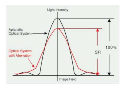
Although RMS and Strehl ratio are different, when the RMS is small they are related by an approximation such that an RMS value of 1/14 wave equates to a SR of .80. Using the relationships between PV, RMS and Strehl, R.F.Royce has produced the following table:
